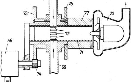
Sept. 26, 1967 APPARATUS FOR PLACING PASTRIES IN PAIRS ONE ON TOP OF THE OTHER Filed June 15, 1965 3 Sheets-Sheet 3
