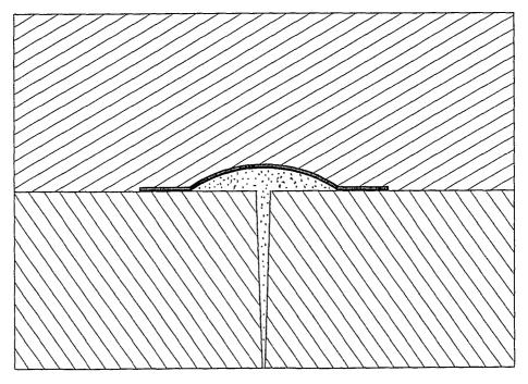
(57) Abstract: Hybrid metal-plastics elements are habitually manufactured by casting/moulding the resin into the rear side of a pressed metal shell. According to the invention, the hybrid element comprising an outer metal skin is manufactured in one step consisting of injection moulding, using the molten injection moulding material as the hydraulic fluid for hydroforming the shell.
