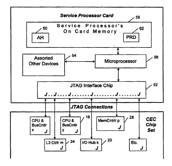
J = JTAG serial interface between Service Processor & chips in CEC
