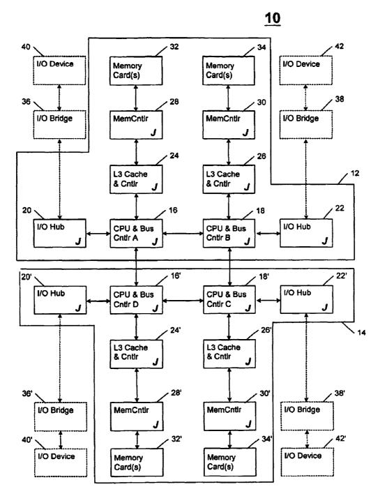
J = chip has serial jtag connection to Service Processor HW ☐ dotted box indicates remote chip or device inaccessible to SP via jtag → dotted line indicates connections to and between remote chips & devices
