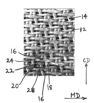
(57) Abstract: A through-air-drying (TAD) fabric for producing tissue paper and related products on a papermaking machine comprising a plurality of warp yarns interwoven with a plurality of weft yarns to produce warp and weft knuckles on a paper-side surface of the fabric, preferably to form an L-shaped knuckle pattern.
