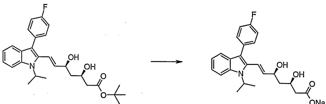
In a 10 ml three-necked round-bottomed flask equipped with a magnetic stirrer, thermometer, septum, syringe and nitrogen supply, 0.49 g of erythro-( $\pm$ )-(E)-7-[3-(4-fluoro-phenyl)-1-isopropyl-1H-indol-2-yl]-3,5-dihydroxy-hept-6-enoic acid tert-butyl ester is hydrolysed according to O. Tempkin, *Tetrahedron* **31**, 10659 (1997), there being obtained 0.35 g (77% of the theory) of a pale beige powder, the NMR of which corresponds to that of the commercial product.
