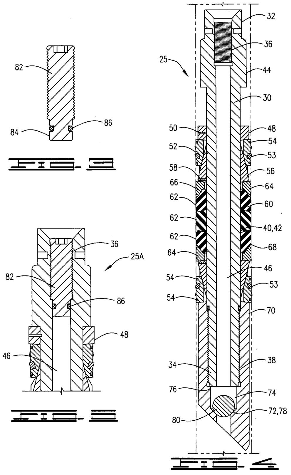
**FRACTURING PLUG CONVERTIBLE TO A BRIDGE PLUG**
