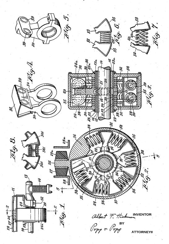
DEVICE FOR PROVIDING TORSIONAL RESISTANCE
