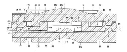
(57) Abstract: Proposed is a variable focus lens package (2) including lens (31, 75) as covers, which covers are provided as moulded replica layers (31, 75) on a substrate (30, 74) and are provided with integral alignment mens (33, 77).
