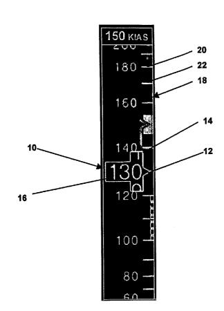
(57) Abstract: A graphical display of a nonlinear scale emulating the view of a mechanical drum gauge. The nonlinear scale may be used for the display of aircraft flight data including airspeed, altitude, heading, and other aircraft data suitable for presentation on a nonlinear scale. The nonlinear scale may scroll to display current aircraft data.
