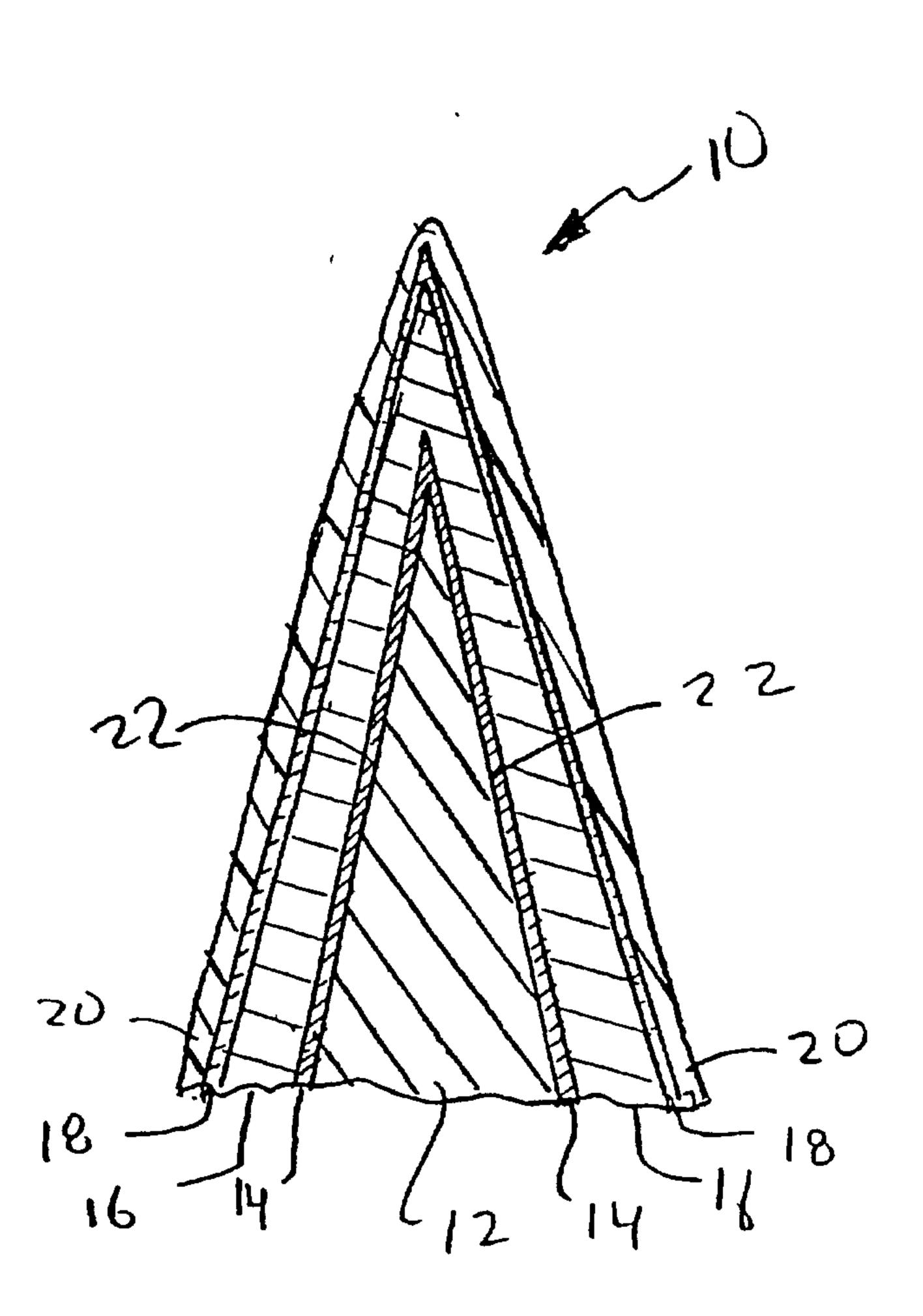
(57) Abstract: A razor blade including a substrate with a cutting edge defined by a sharpened tip and adjacent facets, a layer of hard coating on the cutting edge, an overcoat layer of a chromium containing material on the layer of hard carbon coating, and an outer layer of polytetrafluoroethylene coating over the overcoat layer.
