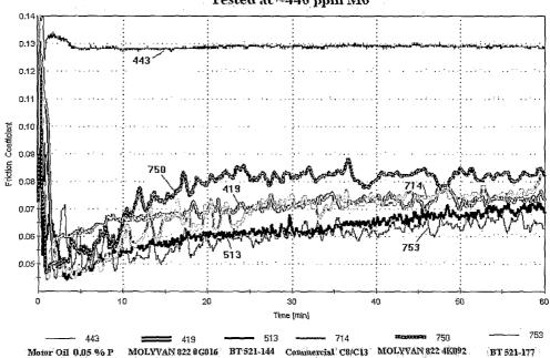
ASTM D5707: 200N; 50Hz; 80°C; 1H; 1mm Stroke; Ball on Disc
