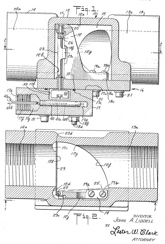
FLOW SWITCH HAVING HIGH SENSITIVITY AT LOW FLOW RATES
