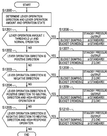
proportional valves 41a, 42a, 42b, 43a, 43b, and 44a and second solenoid proportional valves 41b, 42c, 42d, 43c, 43d, and 44b. The first target pilot pressure correction section and the second target pilot pressure correction section are configured to switch a first standby pressure  $\alpha$  to a second standby pressure  $\beta$  set lower than the first standby pressure in a case in which the standby pressure switching command has been inputted.
