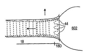
(57) Abstract: A support member for a catheter sheath is disclosed. The support member has a series of ribs with a distal member having integrated fingers for providing radial compliance. The support member provides sufficient axial stiffness to provide a desired pushability of a minimally invasive device Various alternative for replacing a heart valve. embodiments are also described.
