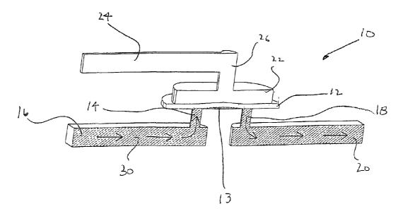
**(57) Abstract:** A pneumatic valve for use in laminated plastic microfluidic structures. This zero or low dead volume valve allows flow through microfluidic channels for use in mixing, dilution, particulate suspension and other techniques necessary for flow control in analytical devices.
