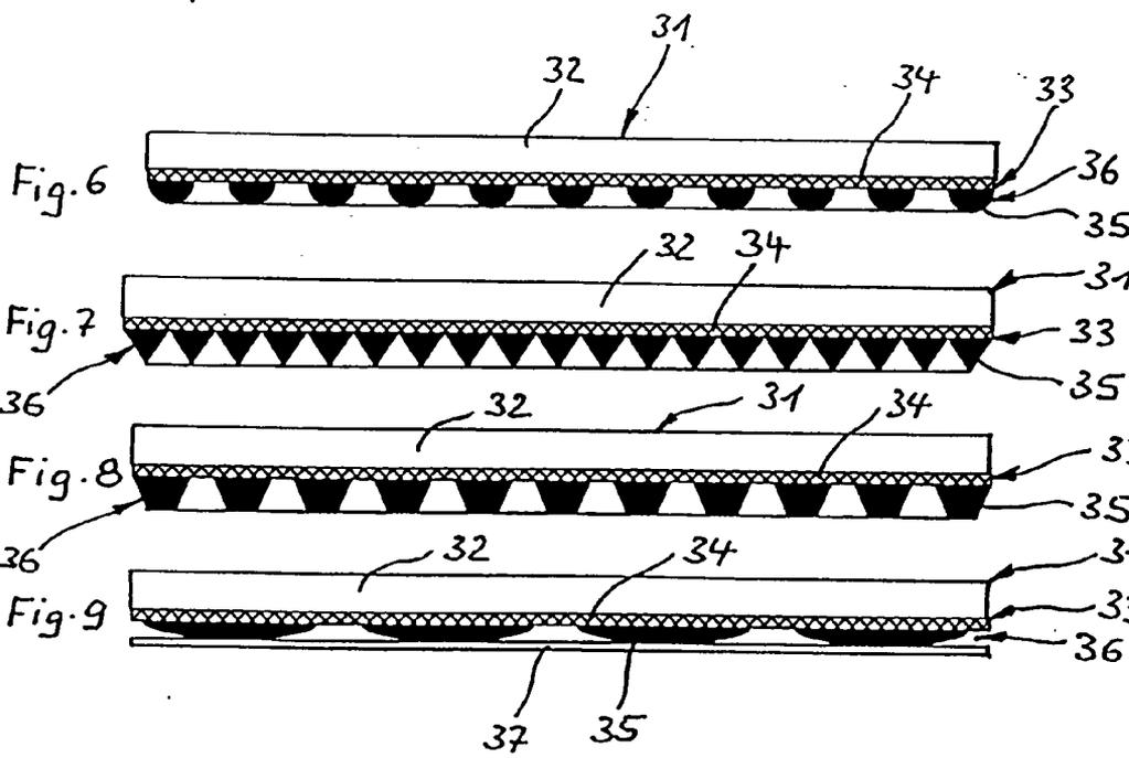
**SOUND-ABSORBING DEVICE FOR A WALL COVERING, CEILING COVERING, OR FLOOR COVERING**
