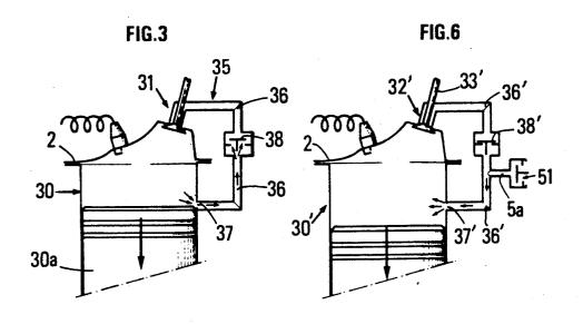
METHOD OF PNEUMATIC INJECTION OF FUEL INTO A CYLINDER OF A RECIPROCATING INTERNAL COMBUSTION ENGINE AND A CORRESPONDING INJECTION DEVICE
