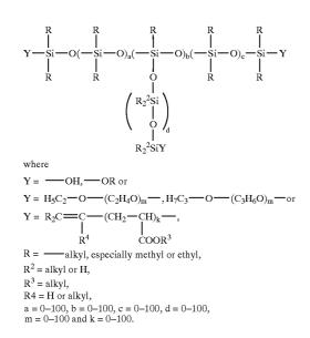
**8**. The coating formulation as claimed in claim 6, wherein the polyorganosiloxane and/or modified polyorganosiloxane is a polyorganosiloxane having the following general structure:
