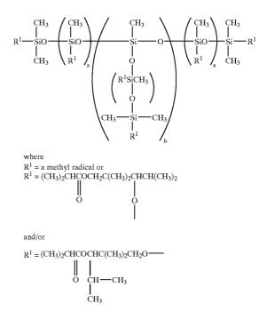
and the sum of the units a=0 to 100, the sum of the units b=0 to 15, the ratio of methyl to alkoxy radicals among the radicals  $R^1$  is smaller than 50:1 and b is >1 if a=0, and a is >5 if b=0.
