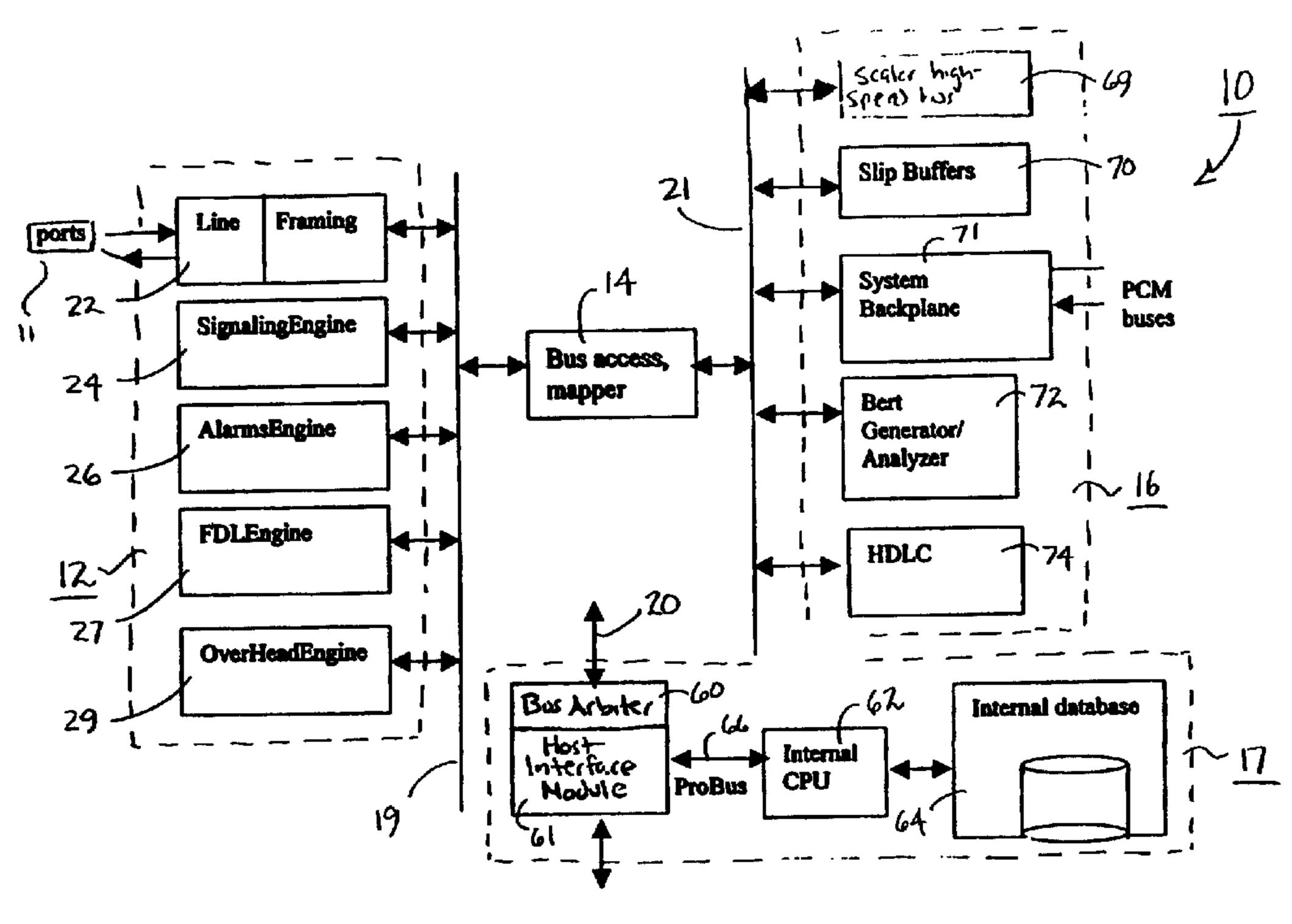
(57) Abstract: A bus framer includes an engine which extracts information from a frame of data being transmitted over a time-division multiplexed bus and a processor which retrieves the information from the engine over an internal bus and forwards the information. The bus framer further includes a mapper which maps the frame of data on the time-division multiplexed bus to a read/write bus and a functional module which receives the data from the read/write bus.
