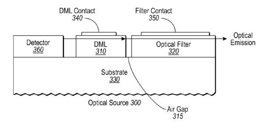
(57) Abstract: An integrated optical source includes a Directly Modulated Laser (DML) and a filter which is positioned with the DML on a common substrate. The filter is configured to receive an input signal in the form of a modulated chirped optical signal. The filter is further configured to provide an output optical signal in the form of an amplitude and/or phase modulated optical signal, optimized for long-distance transmission in optical fiber.
