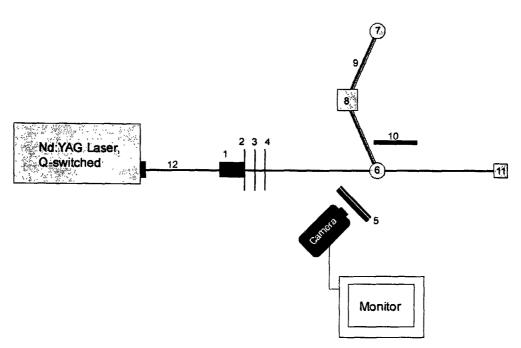
(57) Abstract: A method for the non-photochemical laser induced nucleation in which short high-intensity laser pulses are used to induce nucleation is supersaturated solutions including protein solutions. The laser (12) induces nucleation only in the area (6) where the beam is focused or passes through, resulting in fewer nuclei than would be achieved by spontaneous nucleation. In addition, the laser reduces nucleation time significantly.
