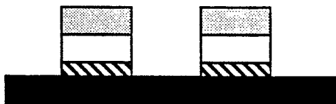
Fig. 3d. The metal layer is now patterned by ion milling using the photoresist-release layer structure as a mask.
