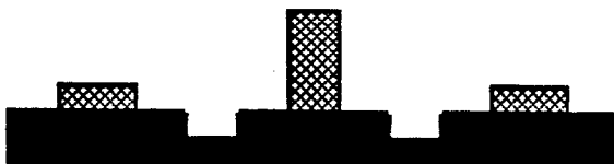
Fig. 2f. The masking structure is removed by dry etching or dissolving the thick planarizing film with an organic solvent.
