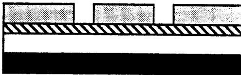
Fig. 1b. The photoresist layer is exposed and developed.
