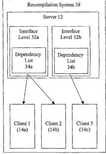
(57) Abstract: An article of manufacture and a method includes providing a system having an interface, dividing the interface into levels, associating a dependency list with a level, associating a client with the dependency list, and marking the clients associated with a dependency list for recompilation based on a change to a global component.
