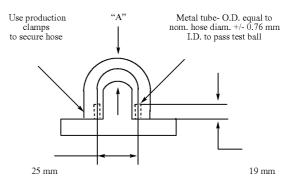
[0048] Sample Selection: Production hose selected for the kink test should represent, as nearly as possible, minimum wall thickness. When recording results include wall thickness, ovality, and dimension "A" (see above). This dimension is measured while sample is on the test fixture.
