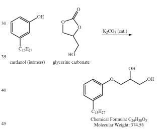
Copolymerization of the polyhydroxylated cardanol derivative with polyacidic monomers in esterification reactions provides polyester polymer resins that have properties similar to those in conventional, commercially available polyester polymer-based toner.
