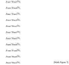
4) For the 361st information bit i360, the addresses of the parity bit accumulators are given in the second row of the addresses of parity check matrix. In a similar manner the addresses of the parity bit accumulators for the following 359 information bits is,  $s=361, 362, \ldots, 719$  are obtained using the Math Figure 6, where x denotes the address of the
