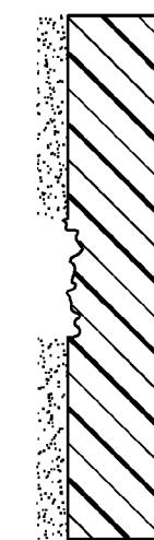
5. Metallization by electroless copper
