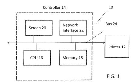
(57) Abstract: A system for creating and/or editing a code for an ink jet printer includes a display screen. A plurality of icons is displayed on the screen. Each icon corresponds to an editable field of a printable code. A plurality of menu items is displayed on the screen. Each menu item corresponds to a property of one or more of the editable fields of the printable code. The printable code includes a lot code or a batch code.
