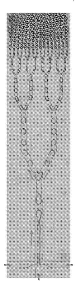
Multiplex Tagman probe fluorescence in drops thermocycle & image nject PCR reagents Split drops Lyse & digest Encapsulated cells in drops with lysis buffer Co-flow with lysis buffer Extremely rare
