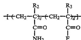
wherein d is a cationic monomer, R<sub>1</sub>, R<sub>2</sub> and R<sub>3</sub> are the same or different and are hydrogen or a lower alkyl group having C<sub>1</sub> to C<sub>3</sub>, F is the salt of an ammonium cation and the molar percentage of c:d is from 95:5 to 5:95 with the proviso that the sum of c and d equals 100%.**13 Claims, No Drawings**
