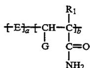
wherein E is the repeat unit obtained after polymerization of an  $\alpha,\beta$  ethylenically unsaturated compound, the molar percentage of a:b is from about 95:5 to 5:95, with the proviso that the sum of a and b equals 100%; G comprises the structure:
