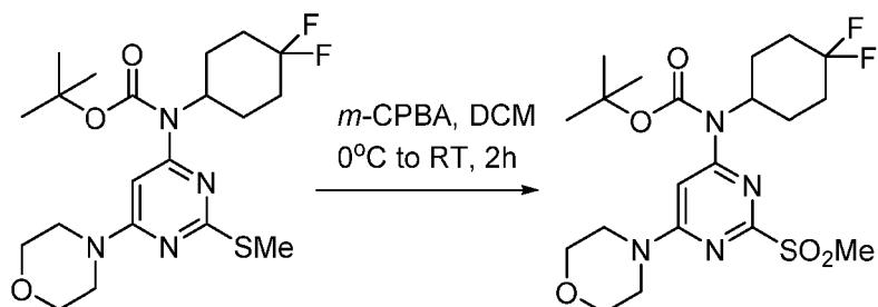
[0074] A 100-mL single neck round bottom flask, connected with reflux condenser equipped with nitrogen gas inlet-outlet U-tube adaptor filled with oil, a teflon-coated stir bar (1 cm), was charged with a solution of tert-butyl (4,4-difluorocyclohexyl)(2-(methylthio)-6-morpholinopyrimidin-4-yl)carbamate (50 g, 112.47 mmol) in dichloromethane (600 mL)
