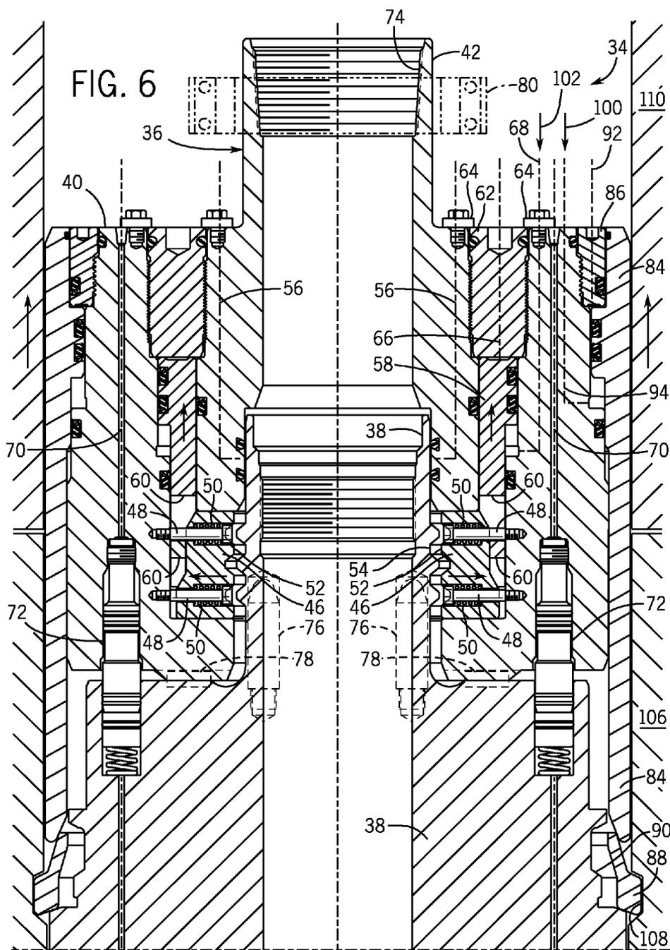
**HYDRAULICALLY ACTUATED WELLHEAD HANGER RUNNING TOOL**
