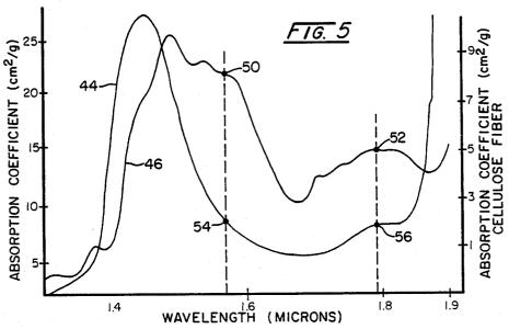
APPARATUS AND METHODS EMPLOYING INFRARED ABSORPTION MEANS TO MEASURE THE MOISTURE CONTENT OF HEAVY GRADES OF PAPER
