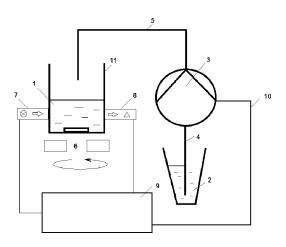
at the micrometering device (3, 4, 5) and the concentration is calculated on the basis of this, where the volume of (2) is much smaller than of (1).
