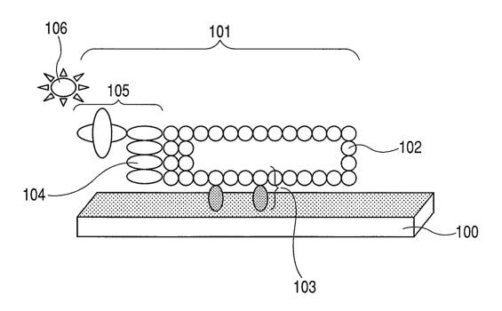
(57) Abstract: It is intended to provide a target substance-capturing body comprising: a base consisting of a soluble protein; and two or more functional domains capable of binding to different target substances.
