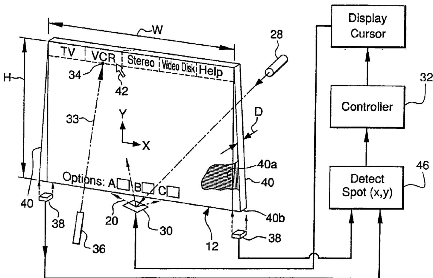
(57) Abstract: A display system includes a waveguide optical panel having an inlet face and an opposite outlet face. A projector and imaging device cooperate with the panel for projecting an image thereon. An optical detector is located near the panel for detecting a location on the outlet face of an inbound light spot. The inbound light is channeled to the detector which may be of a reduced size.
