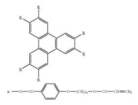
**[0235]** The coating solution was applied on one surface of the polarizing membrane, and dried. Immediately after dried at  $130^{\circ}$  C. for 1 minute to orient the liquid crystal molecules, the membrane was cooled to room temperature and exposed to ultraviolet light in the amount of 500 mJ/cm<sup>2</sup> to polymerize the molecules and thereby to fix the alignment. Thus, a first optically anisotropic (sub)layer (thickness: 1.7 µm) was formed.
