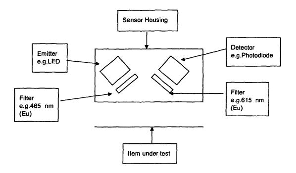
Figure 1: Example of an arrangement for in-situ validation of security label
