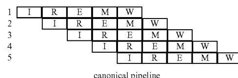
In the diagrams below, we simplify the diagrams somewhat by eliminating the pipe stages for instruction fetch, register file fetch, and register file write, which can be understood to precede and follow the portions of the pipelines diagrammed. The diagram above is shown again in this new format, showing that the canonical pipeline has very little overlap of the actual execution of instructions.
