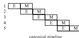
A superscalar pipeline is one capable of simultaneously issuing two or more instructions which are independent, in that they can be executed in either order and separately, producing the same result as if they were executed serially. The diagram below shows a two-way superscalar processor, where one instruction may be a register-to-register operation (using stage E) and the other may be a register-to-register operation (using stage A) or a memory load or store (using stages A and M).
