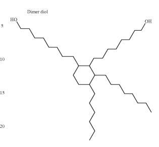
The diol having a cyclic structure and an alkyl chain with two or more carbon atoms is desirably incorporated into the polyurethane resin in a proportion of 5 to 60 mass percent, preferably 10 to 40 mass percent. When the content of diol having a cyclic structure and an alkyl chain with two or more carbon atoms is within the stated range, solubility in solvent is high, good dispersibility is achieved, and durability is good.
