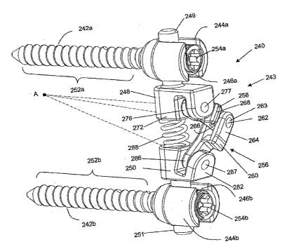
(57) Abstract: A spine stabilization device (240) and methods are disclosed, the device comprising a brace (243) adapted to span between a first bone anchor (242a) and a second bone anchor (242b), the brace (243) including a first member; a second member; wherein the brace (243) allows for movement between the first member and the second member that is restricted to a three dimensional curved path having a substantially constant radius about a center of rotation positioned outside of the brace.
