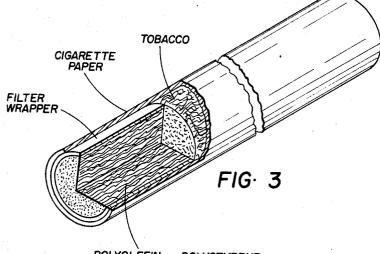
POLYOLEFIN — POLYSTYRENE HIGHLY CRIMPED, FIBRILLATED, AND PLASTICIZER TREATED TOBACCO SMOKE FILTER
