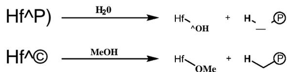
The initial stage of the reaction between TNOA and H<sub>2</sub>O is similar to the reactions shown above for the transition metal-polymer complex. Initial hydrolysis should occur, but secondary reactions will lead to additional hydrolysis reactions (presumably producing AlR<sub>x</sub>(OH)<sub>y</sub> transiently and n-octane), which can then go on to react further to form different
