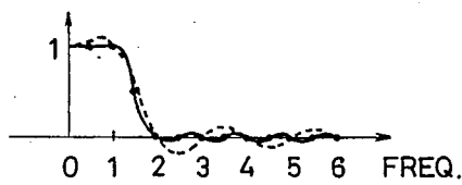
(c) FREQUENCY CHARACTERISTICS OF AN INTERPOLATING FILTER
