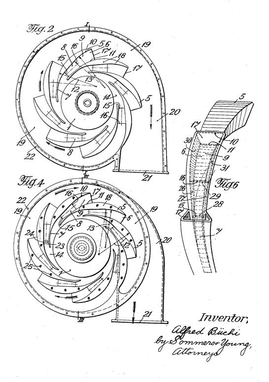
GUIDE APPARATUS FOR CENTRIFUGAL BLOWERS AND PUMPS
