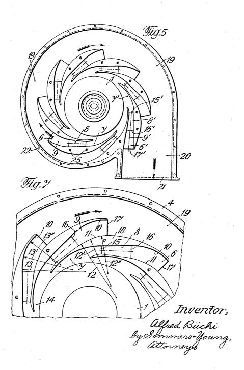
GUIDE APPARATUS FOR CENTRIFUGAL BLOWERS AND PUMPS
