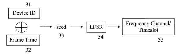
(57) Abstract: A method of operating a wireless mesh network comprises generating a pseudorandom sequence element in a transmitting device and a receiving device of the network using information shared by the transmitting and receiving devices. The pseudorandom sequence element is then used to calculate a communication channel/timeslot assignment for communication between the transmitting wireless device and the receiving wireless device.
