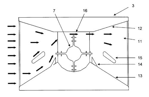
FIG 3 Side Elevation of Turbine Assembly showing current stream flow path
