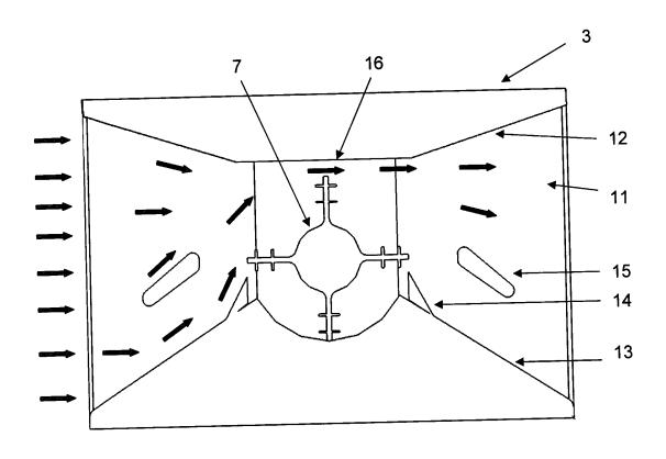
FIG 3 Side Elevation of Turbine Assembly showing current stream flow path
