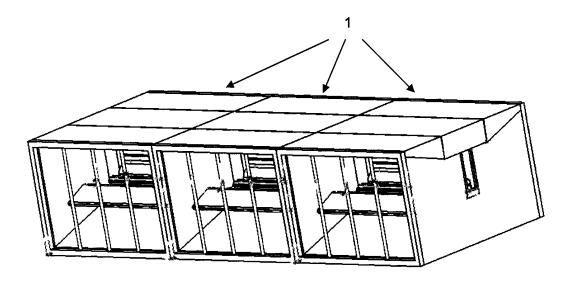
FIG 7 Isometric view of triple bank of horizontal axis turbines
