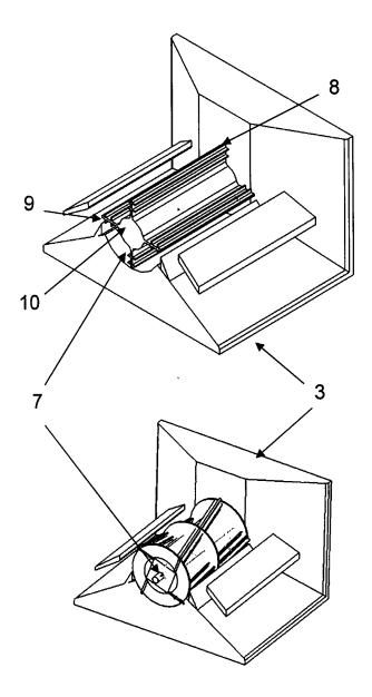
FIG 4 Isometric Sectional View of Rotor Assembly and Flow Guide Profiles
