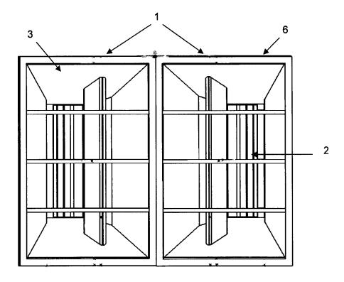
FIG 6 Front View of dual vertical axis turbines
