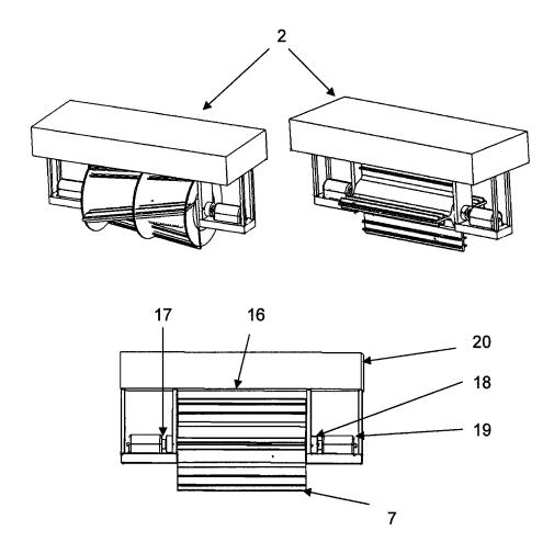
FIG 5 Isometric and Side Elevation View of the Removable Rotor Assembly
