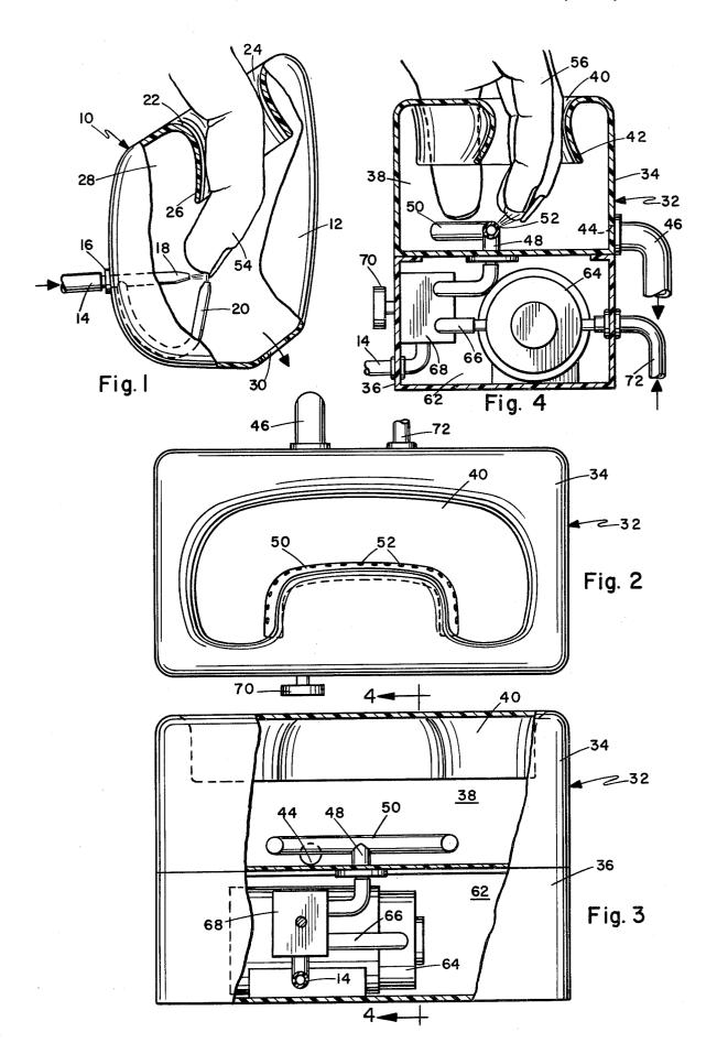
FIG. 1 is a side elevation view, partially cut away, of one form of the fingernail cleaner.
