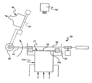
at an outlet en face (104) of the honeycomb body (100) through defects, if any, in the honeycomb walls and/or plugs and passes through a permeabl member (28), such as a screen, where they are illuminated. The permeable member (28) is disposed adjacent to and preferably in contact with the outlet end (104). Use of the permeable member improves the signal-to-noise ratio (SNR) such that defects may be more readily detected. The permeable member (28) preferably includes an anti-reflective surface.
