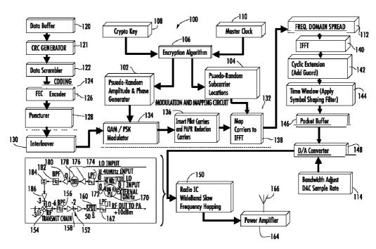
(57) **Abstract:** A system and device communicates data A modulation and mapping circuit modulates and maps data symbols into a plurality of multiple subcar $\pi$ ers that are orthogonal to each other based on a fixed or variable symbol rate A frequency domain spreader circuit is operatively connected to the modulation and mapping circuit and spreads the multiple subcar $\pi$ ers over the frequency domain
